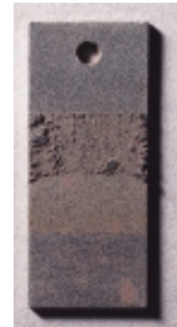
CEMENT-METAL (CM) One-coat system
